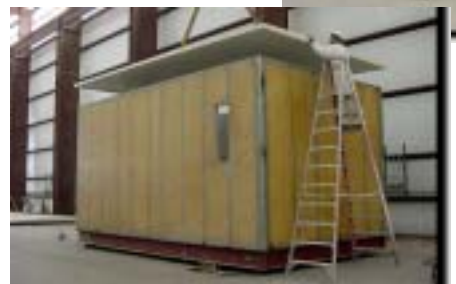
Bebco Shelters are assembled step, by step, from individual wall & roof sections, following an initial coating application
